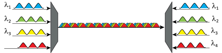
Figure 7: SWDM combining four wavelengths from 850 nm to 940 nm
